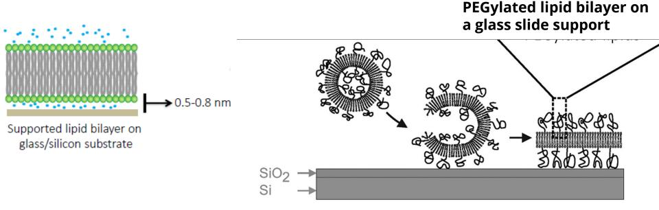
**PEGylated lipid bilayer on a glass slide/silicon support.** Vesicles with PEG are formed, broken and eased onto a silicon substrate for single molecule experiments on ClyA. The PEGylation was done in the first place to lift the lipid bilayer over the substrate to provide room for ClyA to insert into the membrane completely,
