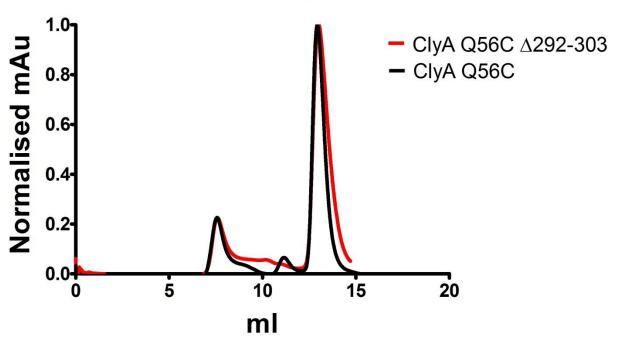
• Gel Filtration profiles for both the wild type and the mutant protein show a single broad monomeric peak at around 14 seconds, indicating no aberrant aggregated proteins formed due to the mutations. The curves were normalized with the maximum mAu of the individual curves obtained.
