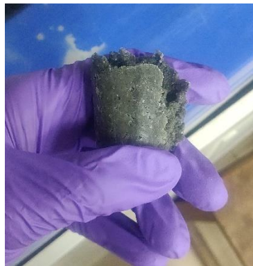
M-sand and PMMA treated sample
