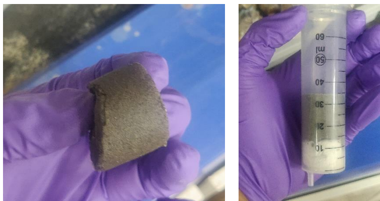
M-sand and epoxy resin samples at varied concentration
