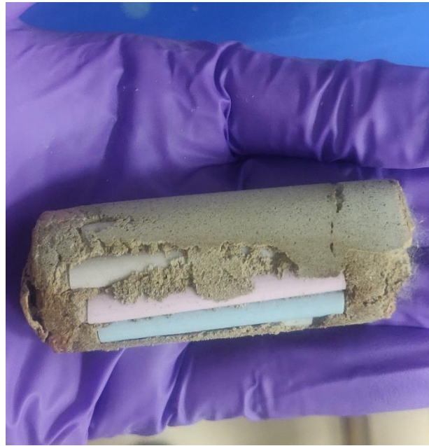
Sand containing straws axially inoculated with bacteria
