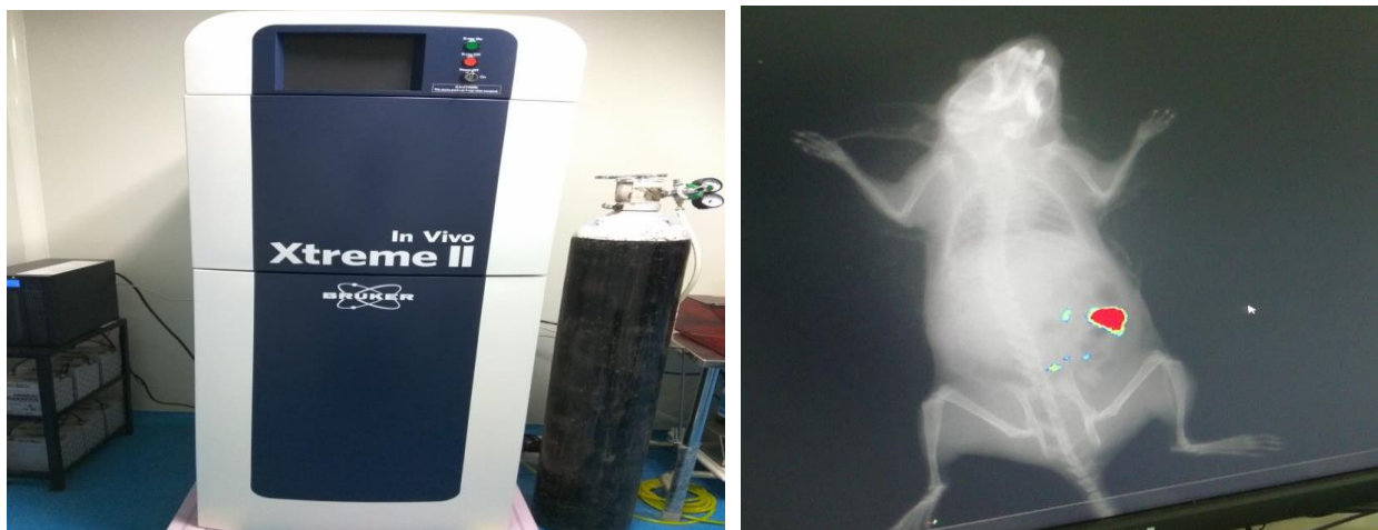
[Figure 8: In Vivo Xtreme imaging equipment (left) and X ray, fluorescent and bioluminescent imaging of a C57BL/6 black mouse (right)]
