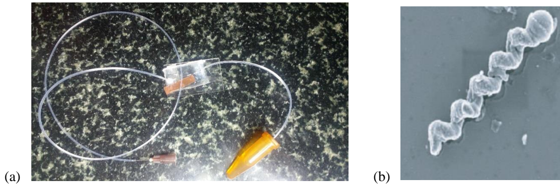
Figure 4: (a) Microfluidic chamber used for flowing nanopropellers (b) SEM Image of a single nanopropeller. [1]
