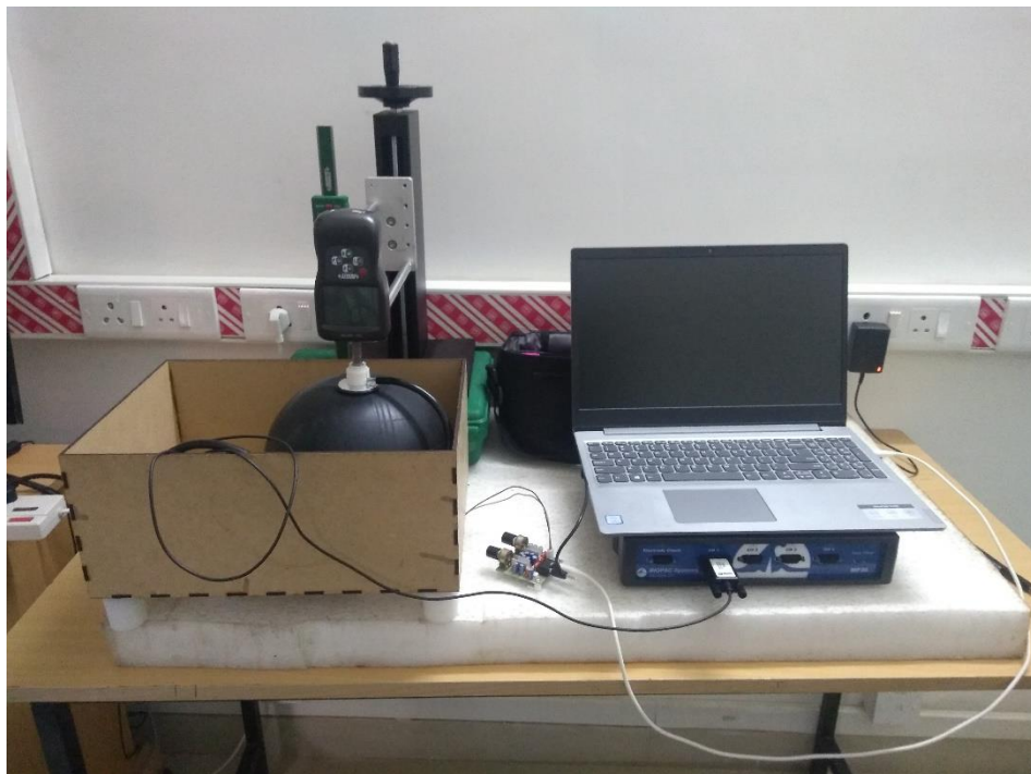
Figure 9: Experiment Setup using a foam (~6cm height) at the base of the setup to reduce the vibrations reaching the sensor.
