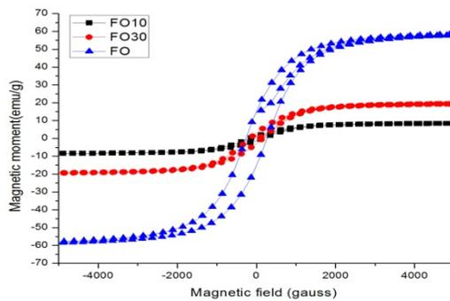
**Figure 11. Plot showing hysteresis loop of different samples analysed by VSM.**
