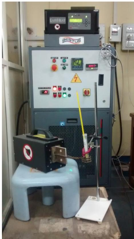
**Figure 5.** alternating magnetic field apparatus.
