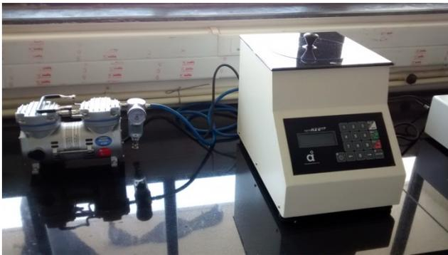
**Figure 1.** Spin coating machine.
