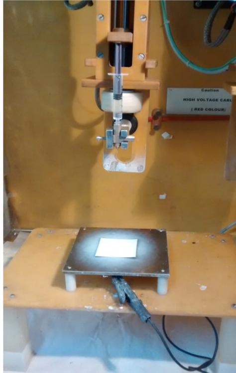
**Figure 2. Electrospinning machine.**
