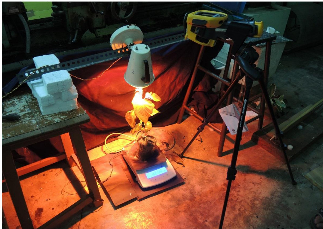
Fig 5. Temperature variation of three points on three different leaves of a plant on which IR radiation from a 150w lamp is incident.
