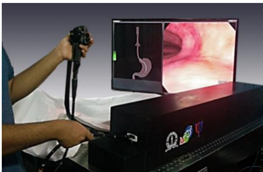
The endoscopy simulator with instrumented endoscope, developed in IISc and incubated by Mimyk
