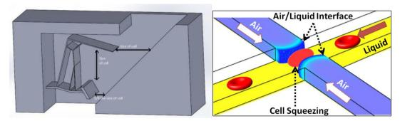
Conceptual design of movable solid-liquid and air-liquid interfaces to test the deformability of single RBCs in flow
